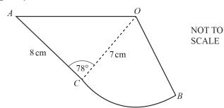
The diagram shows a design made from a triangle AOC joined to a sector OCB. AC = 8 cm, OB = OC = 7 cm and angle  $ACO = 78^{\circ}$ .
