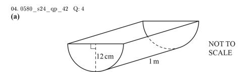
The diagram shows a tank in the shape of a half-cylinder of radius 12 cm and length 1 metre. The tank is fixed horizontally and is completely filled with water.
